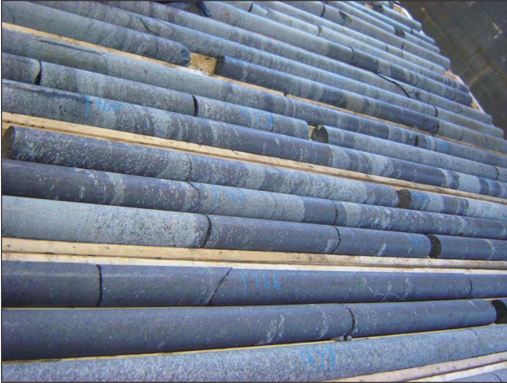
Figure 8-2: View of the Footwall Massive Magnetite Units
