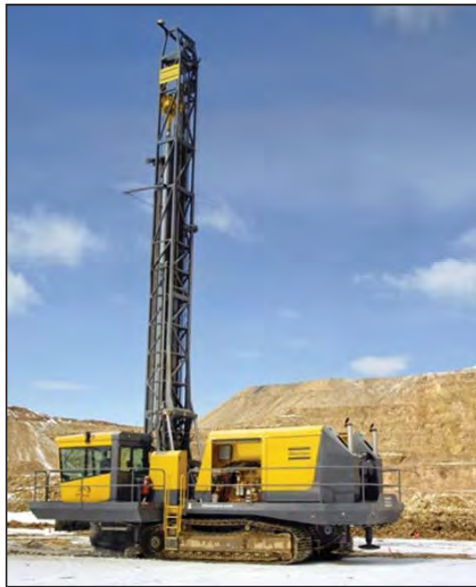
Figure 16-22: Rotary Tower Drill Atlas Copco Viper 235
