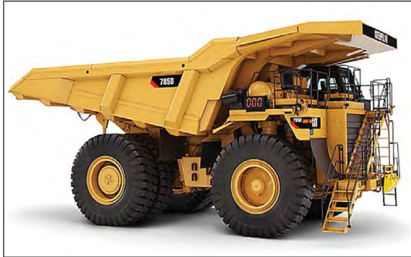
Figure 16-28: Hauling Truck CAT 785D (140 tonnes payload)
